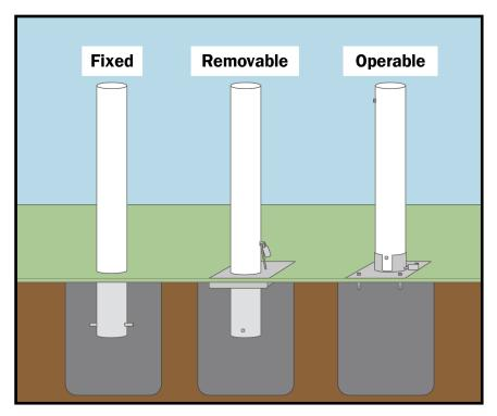
**Figure 8.** Rated bollards comprised of metal posts supported by foundations designed and tested to mitigate vehicle rammings. Ensure proper engineering and anchoring of bollards by qualified professionals, and inspect and maintain devices at manufacturer-identified intervals.
