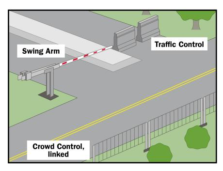
**Figure 9.** Barriers for perimeter protection, dividing secure areas from public access or at entry gates to control access.
