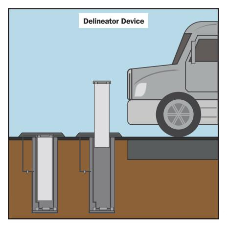
**Figure 7.** Delineator devices may be unrated and have limited potential to stop an approaching vehicle.
